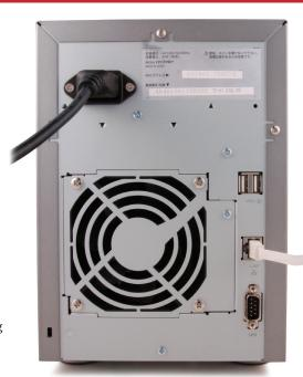
Begin setting up your TeraStation by plugging your *power cable* and *Ethernet cable* into the back of the TeraStation as shown.
